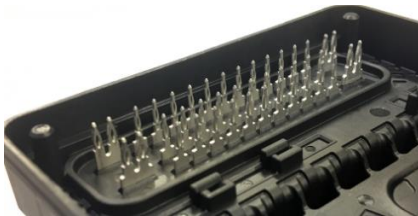
Figure 1 – Press-Fit in Brake Module
