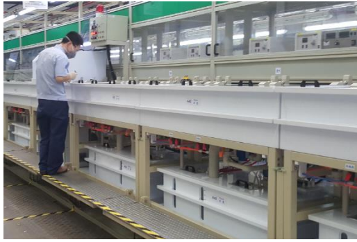
Figure 3 - Reel-to-reel Plating Line
