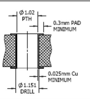
PCB Hole Construction for Interplex's 0.64mm Press-fit Section
