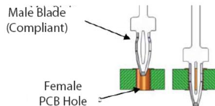
Normal Force is the force exerted on the walls of the PCB hole by the spring characteristic of the press-fit pin. Insertion Force is the force exerted back against the pin when inserted into the PCB. Because press-fit joints on PCBs are more permanent than blade-and-socket connectors, which are designed to be disconnected and reconnected, the PCB to press-fit terminal interface needs to have much higher Normal Force after insertion.
