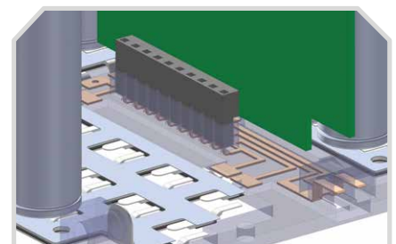
Female receptacle connects control board to overmolded lead frame male connector
