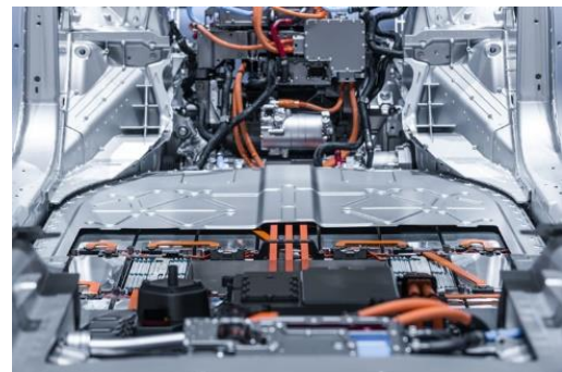
Figure 1 - EV Lithium Battery Module
