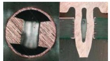
Direct Connect to PCB hole (no solder voids)
