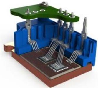
Wire Bond to Press-fit Power Module
