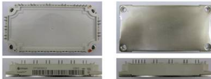
Figure 2 – Example Heat Sinks on Power Module
