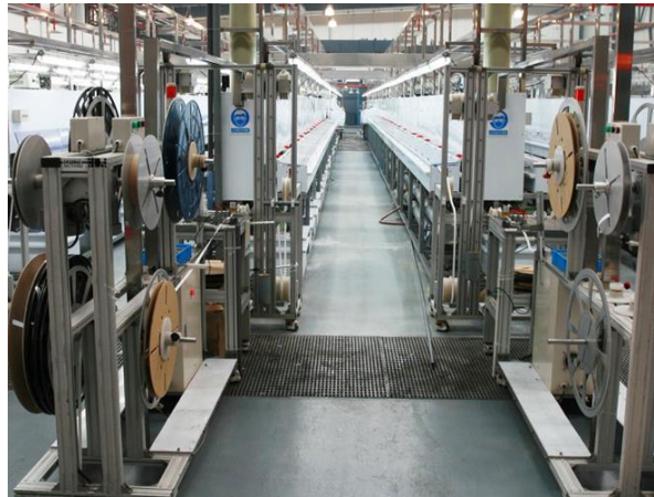
Figure 2 - Reel-to-Reel Plating Production Line
