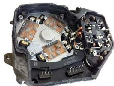
Figure 1 – EPS Power Control Assembly
