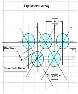
If we increase our X-Pitch to 0.160 mm, our Y-Pitch 0.1386 mm and our Hole Density reduces to 4511 holes per square centimeter.
