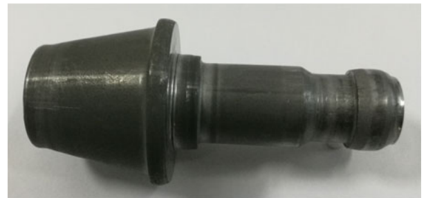
Figure 2 - Cold Forged Part
