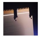
Selective Brush Plating – provides a cost effective method of applying selective plating to continuously reeled parts using a brushing method. Brush plating is typically a post-stamping process and can be very cost effective for plating of specific features such as the raised contact areas shown at right.
