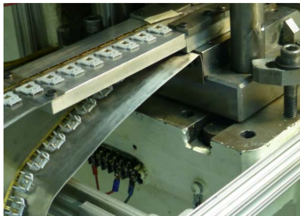
Two Dissimilar Strips – Stitched Together
